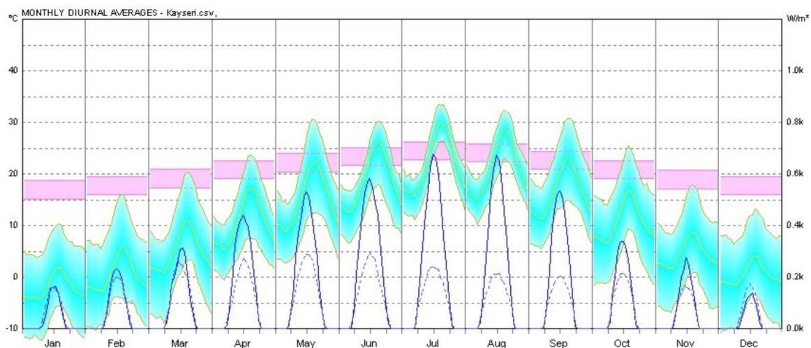
*Figure 3: Diurnal range of outdoor air temperature (green bands) and solar radiation on a horizontal surface (values of direct radiation shown by solid blue lines and diffuse by broken lines) for Kayseri plotted against thermal neutrality bands (shown in pink).*
