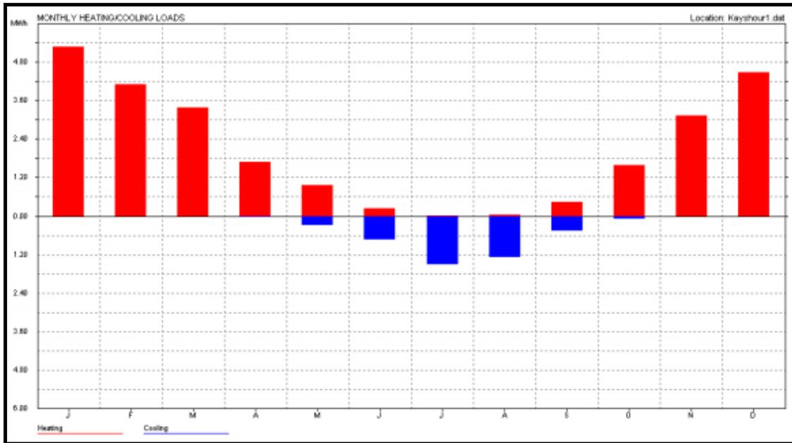
Figure 18: Monthly Heating/Cooling Loads of Basturk House with Mud-Brick Walls.
