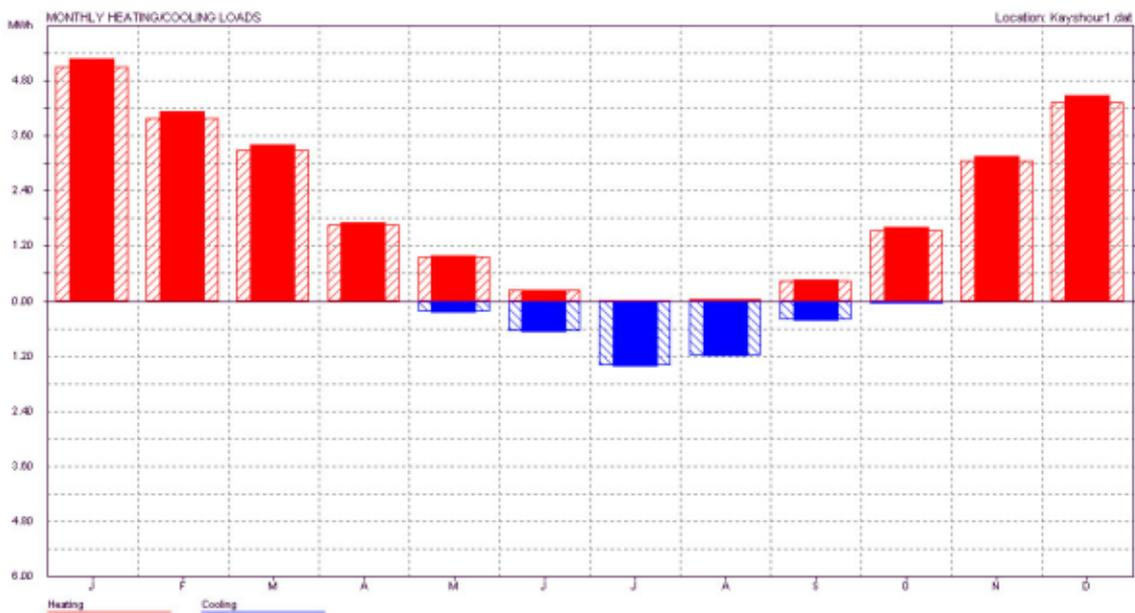
Figure 22: A Comparative Graph Showing Monthly Heating/Cooling Loads of Basturk House with Hollow-Brick-Insulation and with Mud-Brick Walls. Hatched Bars Showing the loads with Hollow-Brick Walls with Insulation and Solid Bars Showing the loads with Mud-Brick Walls.
