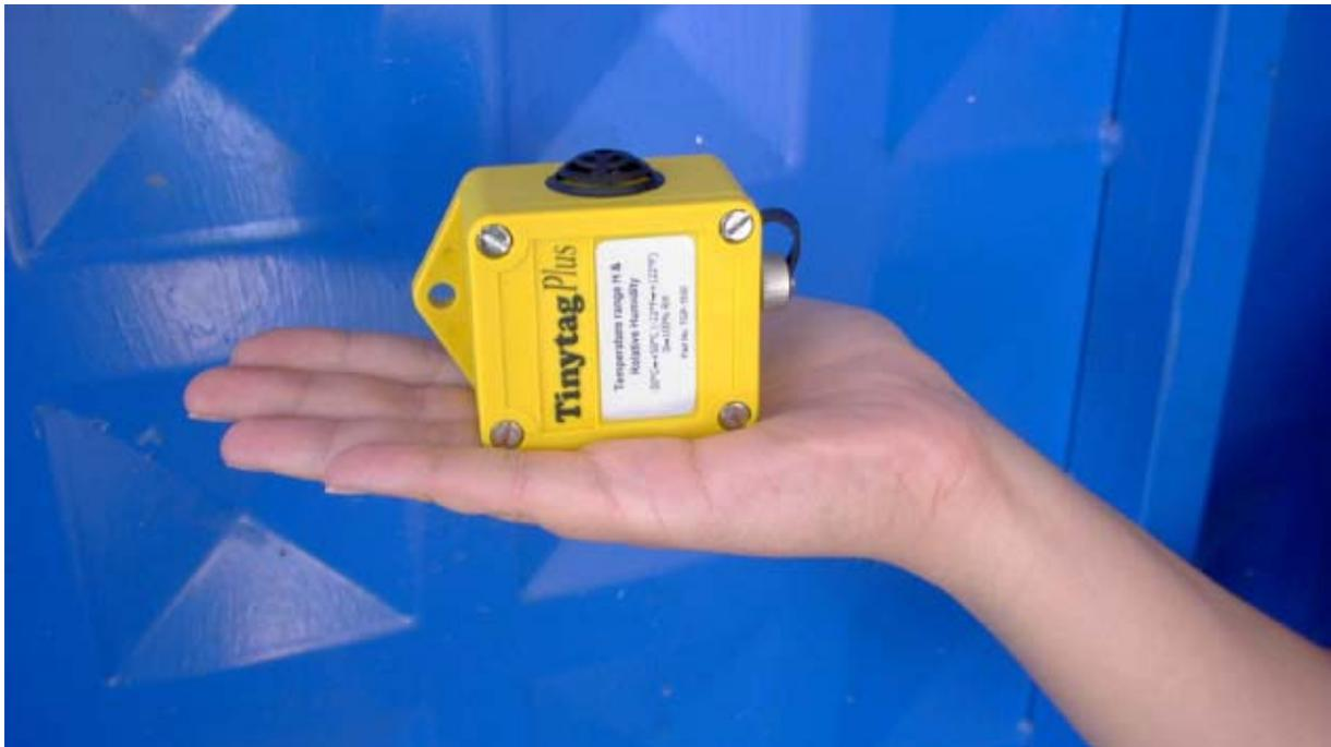
*Figure 5: Tinytag data logger with the sensor protected by a black spherical frame.*
