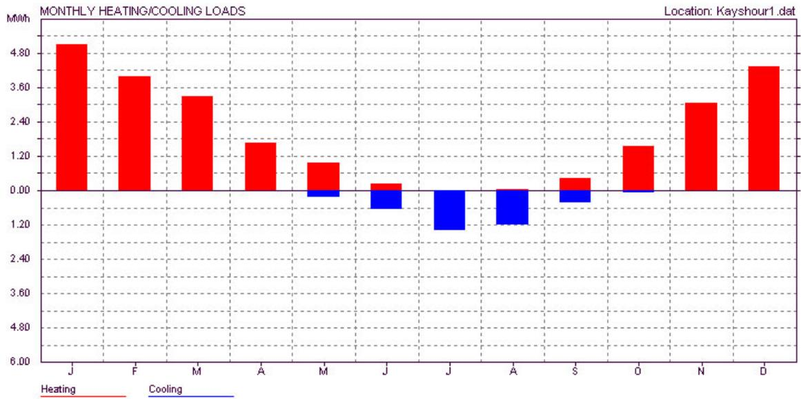
Figure 19: Monthly Heating/Cooling Loads of Basturk House with Hollow Brick Walls with Insulation.
