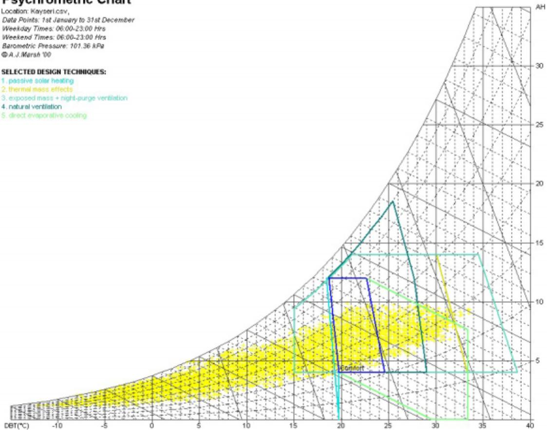
Figure 4: Hourly data for a Kayseri year plotted against thermal comfort zones on psychrometric chart (Source: Meteonorm and Weather Tool software).
