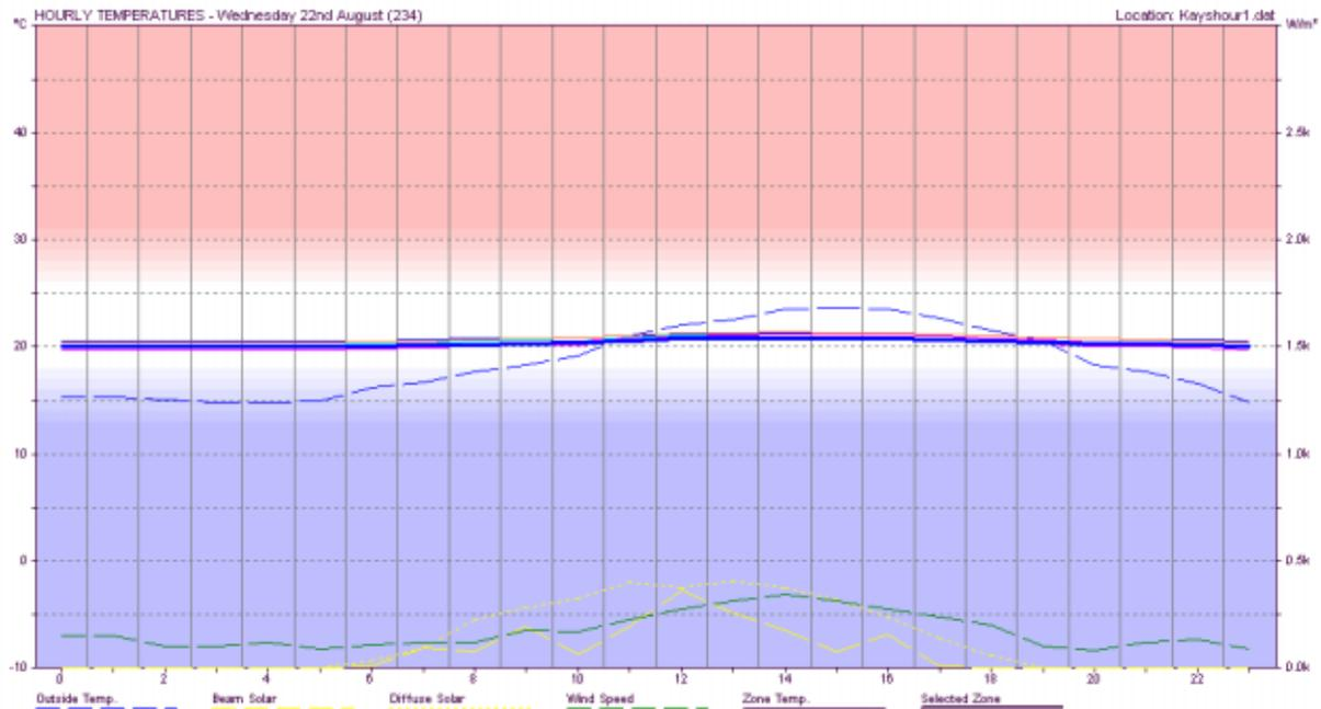
*Figure 23: Graph Showing the Hourly Temperature Distribution of Babayigit House with Stone and Mud-Brick Walls. (23rd of August).*
