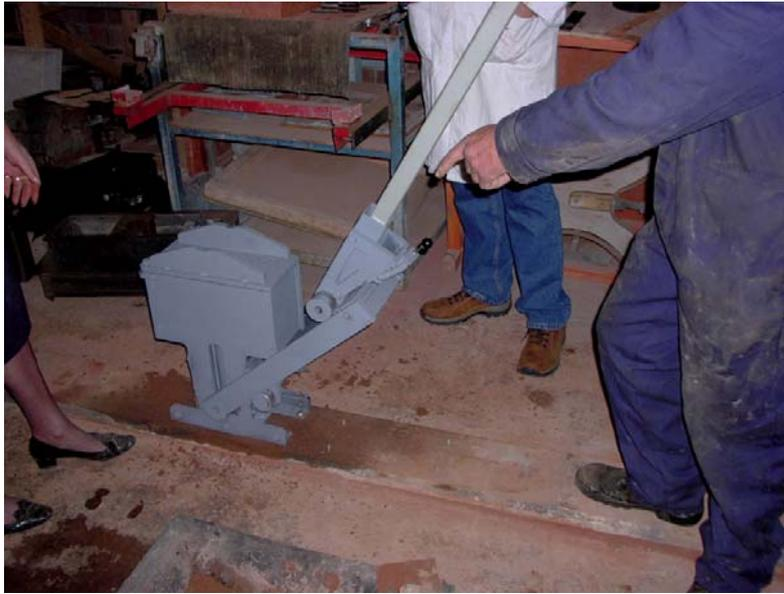
*Figure 4. Pressure is applied to the mixture of clay, sand, cement and water in the Parry's Brick Press mould by means of a long handle.*
