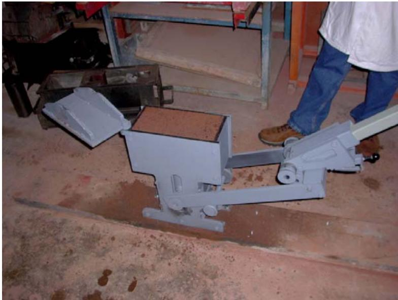
*Figure 5. The lid of the brick press is opened and the brick pushed up as the handle is released.*
