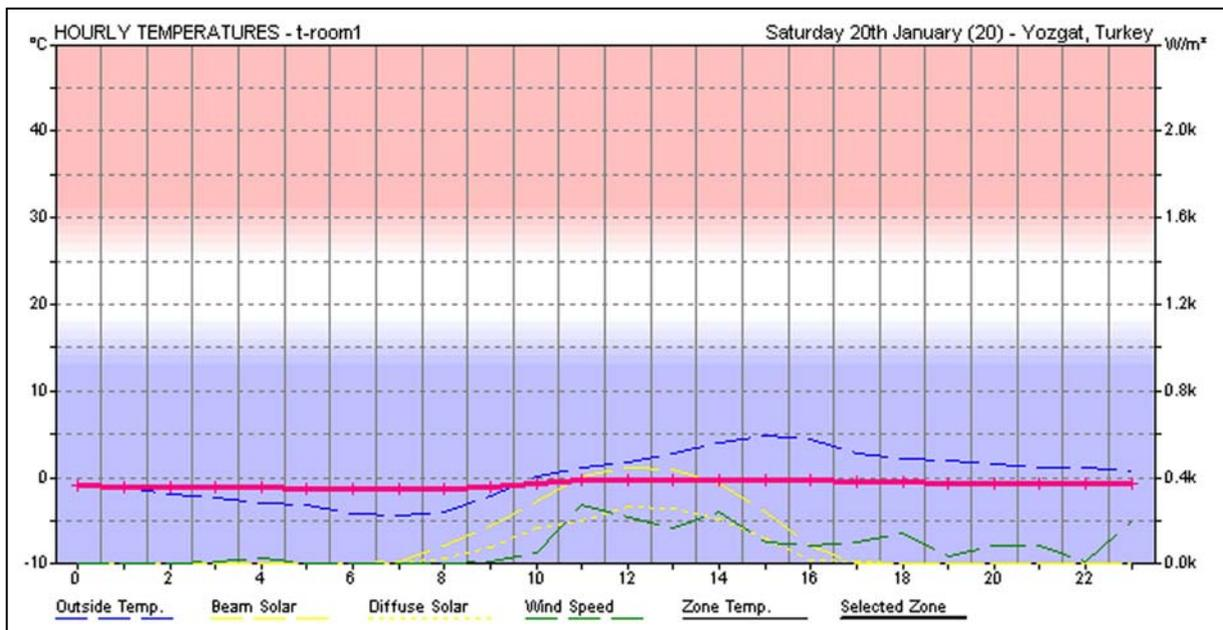
Figure 21. Hourly temperature profile inside the mud-brick building (pink line) on the 20th of January 2004 compared with weather data (5 years average) for Yozgat displayed in Ecotect v.5.20.
