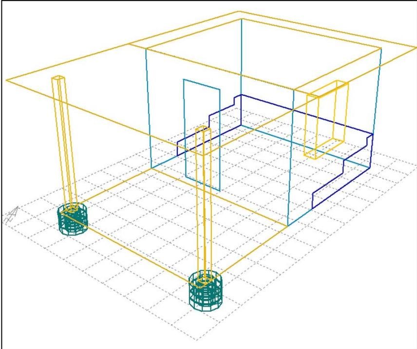
*Figure 17. A 3D view of the thermal model of mudbrick building developed in Ecotect v.5.20.*
