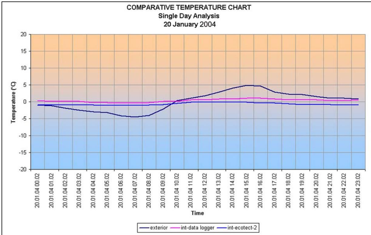
Figure 20. Comparison of hourly temperature profiles for a single day analysis (20 January 2004) obtained from interior datalogger (pink line) and profiles obtained from computer simulations performed in Ecotect v.5.20 (blue line). Air temperature recorded by exterior datalogger (dark blue line) is also given here.
