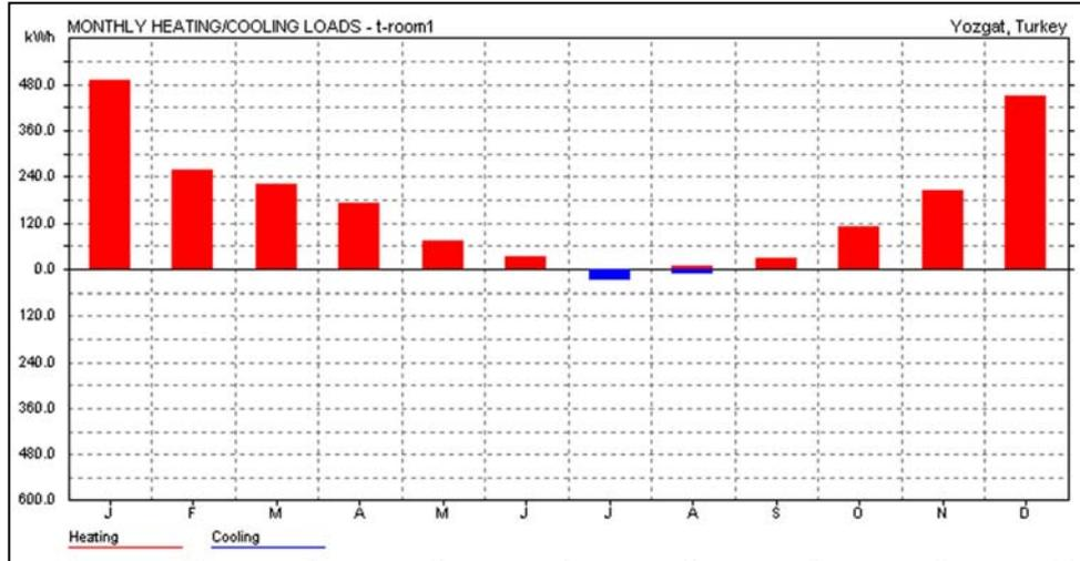
Figure 22: Monthly heating and cooling loads of an air-conditioning system assumed to be located in the mud-brick building as calculated by using thermal analysis function of Ecotect v.5.20.
