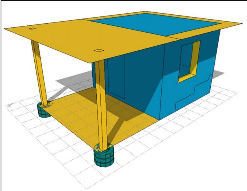
*Figure 18. Captured view of the rendered thermal model with shade and shadows as calculated with Ecotect v.5.20.*
